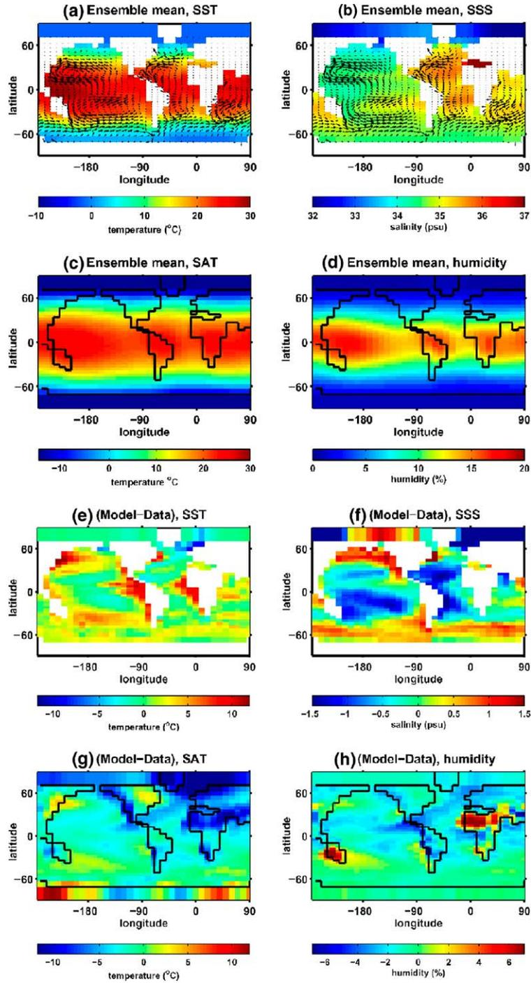
Fig. 1. (a–d) Ensemble mean surface ocean and atmosphere: SST = sea surface temperature; SSS = sea surface salinity. (e–h) Difference between the model ensemble mean and the data used for the assimilation, for the variables shown in the upper plots.
