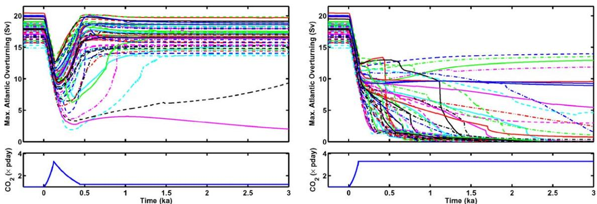
Fig. 7. Sensitivity of the fate of the THC to  $\text{CO}_2$  recovery rate. Maximum Atlantic overturning for ensemble RTP for  $3.3\times \text{CO}_2$ : left plot—with fast  $\text{CO}_2$  recovery; right plot—stabilisation at  $3.3\times \text{CO}_2$ .
