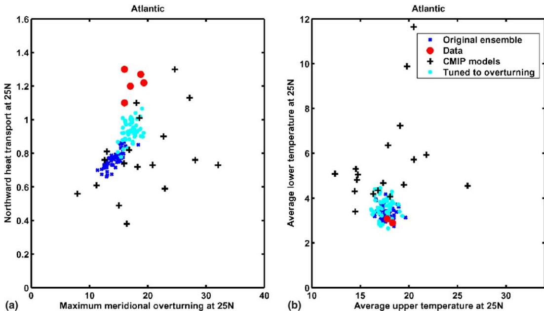
Fig. 2. Comparison with Coupled Model Intercomparison Project, Jia (2003). Dark blue crosses are the original tuned ensemble; cyan crosses are the ensemble with re-tuned THC; black crosses show the results from the CMIP project; red dots are the observational data (Jia, 2003).
